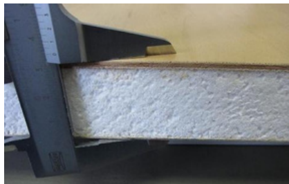
Example sandwich: aluminum - insulation - plywood
