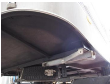
Caravan floor: massive flake board, little protected
